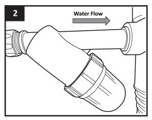
**IMPORTANT:** Before connecting ensure your tanks water outlet is closed off. Connect the Y-Strainer between your tanks water outlet and the pumps suction inlet. Position the filter so that the arrow on the body points in the direction of the water flow. Ensure that there is at least 100mm between the filter and pump to allow the filter to be removed for cleaning.
