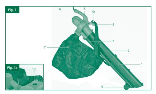
First fit together the front suction tube (1), the rear suction tube (2) and the rear blower tube (3) Then screw the tubes together using two of the longer screws (11) provided. Finally, fit the suction tube assembly into the motor housing and affix them in place with the one long screw (11) and with one short screw (12) on each side.
