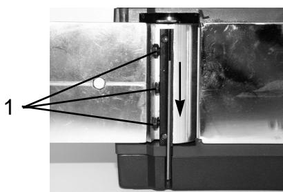
Clean the blade bed before inserting the blade.
