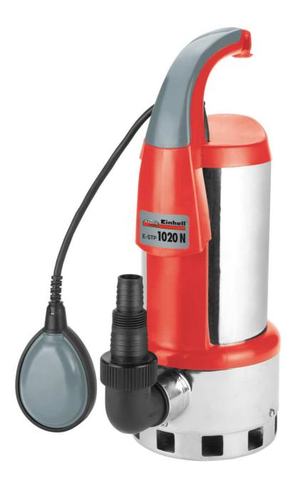
The rugged and powerful submersible sewage pump for moving waste water, it takes foreign particles up to Ø 20 mm in size. In addition to its typical use in excavation pits, this pump is particularly suitable for emptying garden ponds and swimming pools. Thanks to its continuously adjustable float switch the pump is an indispensable tool during floods and in case of burst pipes.
