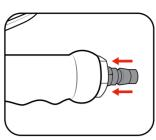
4. Pull back the sleeve on hose fitting, insert male end & release sleeve on hose fitting.
