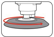
2. Press the sand paper onto the sanding pad, making sure to align the edges.
