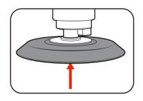
3. To remove the sand paper, peel off starting from one edge.
