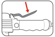
3. To adjust the rotational speed of the sander, rotate the air regulator dial until the desired setting is achieved.
