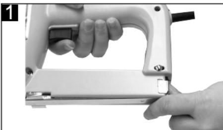
Pull the magazine slide out of the back of the electric stapler/nailer (Fig. 2).
