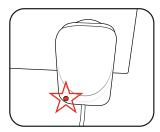
With the battery sitting on a flat surface, align the raised ribs on the battery with the recess in the charging cradle and slide onto the battery ensuring a firm connection.
