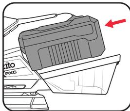
2. To remove, hold down the battery release button and then slide the battery out.
