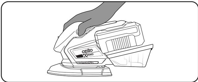
3. Gradually lower the sander onto the workpiece with a slight forward movement.
