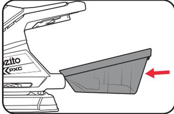
2. To remove, simply pull the dust canister away from the sander.
