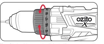
Note: Selecting a higher torque setting will allow the drill to use more torque to drive the screw in or out. To prevent damaging the screw head, it is recommended to start at a low torque setting and increase when necessary.
