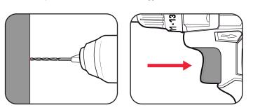
6 Move the drill bit into the workpiece.
