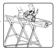
4. Withdraw the chainsaw from the cut while the chain is still running.
