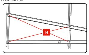
Once all the legs and cross struts are joined together and the fasteners are assembled, use a spanner and screwdriver to tension the fasteners to complete this half of the structure. 7. Repeat the exact process, steps 1-6 for the other side, however leg C is positioned off centre to the right, this will allow correct alignment with the first half when joining them together.
