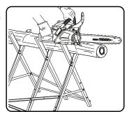
3. If you cannot cut the timber in a single stroke, apply light pressure to the front handle and continue sawing, draw the chainsaw back a little then apply the bucking spikes a little lower and finish the cut by raising the rear handle.
