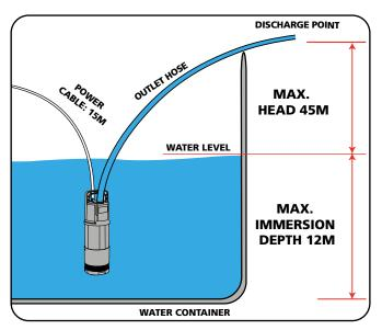
Ensure the pump is placed on a flat and level surface, there are no obstructions to the suction base and it is clear of mud or sediment.
