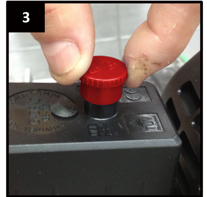
3 To start the unit, pull the On/Off switch upwards.
