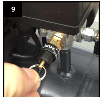
9 Release the pressure in the tank by pulling the safety valve.
