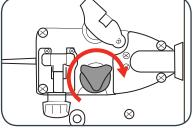
**Note:** Do not over tighten the drive roller bracket as this could damage the MIG welder.
