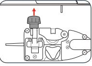
2. Pull the pressure screw arm down and raise the pressure arm.
