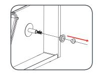
3. Slide the welding wire coil onto the shaft.
