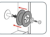
4. Align the spring and drive washer lug with the slot in the drive shaft and secure with the retaining nut, but do not over tighten.
