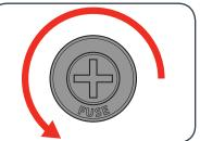
2. Remove the fuse from the holder and replace if the fuse has blown. Refit the fuse holder by rotating clockwise.
