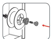
**Note:** Over tightening of the retaining nut will restrict the wire feed rate and can cause damage to the wire feed motor or irregular welding.
