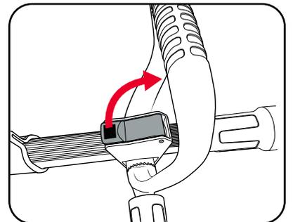
2. Slide the handle into the desired position and then lock in place with the lever.
