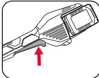
3. To stop the trimmer, release the trigger.
