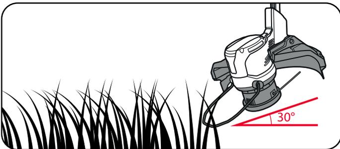
Use only the tip of the cutting line to do the trimming especially near walls and fences. Trimming with the side of the cutting line may overload the motor, wear out the line faster, and break the line more often.
