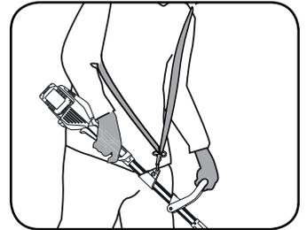
3. To turn on squeeze the variable speed trigger whilst holding the safety switch forward.
