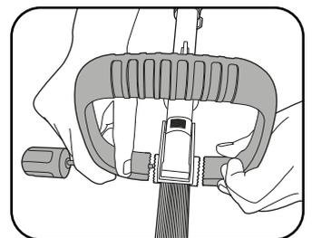
2. Place the adjustable handle on the mounting bracket, then pass the screw with washer through the handle and onto the mounting bracket.
