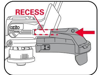
3. Slide the safety guard in place and secure with the socket head bolt. Tighten with the hex key.
