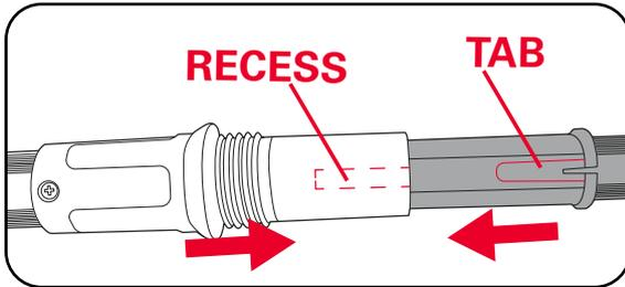
2. Screw tight with the shaft lock collar.
