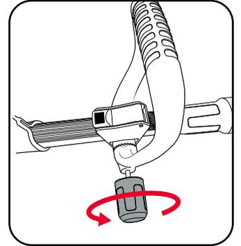
2. Rotate the handle into the desired position and tighten the knob to lock in place.
