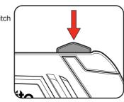
2. Slide the switch forward so that the bit is pushed into the bit holder
