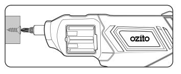
Note: Do not force the screwdriver or apply side pressure to elongate the hole. Let the screwdriver do the work.
