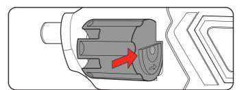
2. Push the cartridge into the screwdriver until it clicks into place
