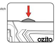
2. Slide the switch backward so that the bit retracts from the bit holder
