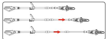
3. To lock in the desired position, twist the telescopic tube lock in a counterclockwise direction.
