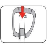
2. Pass the bolt through the auxiliary handle and screw the lever to the end of the bolt
