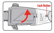
. The pruner head will lock onto the motor head and is then secured in place.
