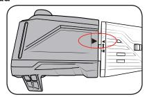
. (a) Press the pruner head against the motor head. This will cause the lock button to be pushed to the (b) Turn the pruner head clockwise. The pruner head will lock onto the motor
