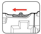
3 If plunge cutting, use a slight pendulum motion.
