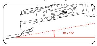
Note: Allow the scraper to do the work; do not apply heavy pressure to the multi function tool. This may cause the multi function tool to overload or cut into the surface of the workpiece.
