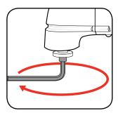
2 Place the accessory onto the spindle making sure to align the accessory with the pins on the spindle.
