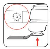
3 Screw the washer and hex screw into the drive spindle and tighten with the hex key to secure the accessory in place.
