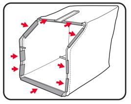
3. Pull the rubber clips over the metal catcher
