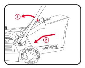
**WARNING!**: ONLY FIT AND REMOVE THE GRASS CATCHER WHEN THE SCARIFIER IS SWITCHED OFF AND THE MOTOR HAS COME TO A STOP.
