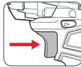
2 Check the forward/reverse lever is on desired setting.
