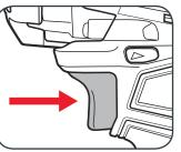
6 Slowly increase pressure on trigger to appropriate torque for circumstances until screw or bolt is tightened.
