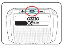
2. Press and hold down the power button again to turn the speaker off; the power button LED will go off.
