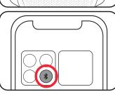
**Note:** Only 1 device can be paired via Bluetooth at any time. Turn off Bluetooth on the first connected device to pair a new device with the speaker.
