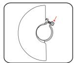
Tighten guard nut then close the guard lever.
