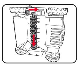
3. To fit the roller, push the roller in the square-ended drive. Push the other end into the scarifier and close the lock.
