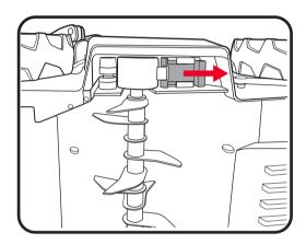
1. To remove the roller, push the roller lock to the right, front of the Scarifier to unlock.
