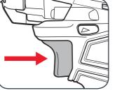
3 Control the speed by adjusting the amount of pressure applied to the
