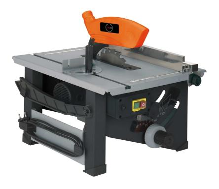
The NTK 900 table saw has been designed for multi-purpose applications including ripping and crosscuts of lumber, chipboard, plywood, multiplex board and veneered board. The saw can be tilted up to 45° for mitre cuts. Thanks to its compact construction the circular saw is ideal for mobile applications. The parallel stop with two stopping heights guarantees precise cuts.
