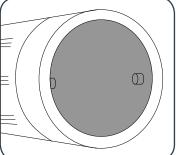
3 Line up the internal nozzle nodes with the blower housing and slide into place.
