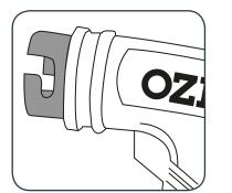
Both the blower nozzle and central inflation adaptor are fitted with internal nodes that line up and slot into the blower housing.
