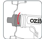
4 To fit inflation adaptor to a small inlet, use either of the other 2 adaptor ends. Fit larger end of smaller adaptor piece to central adaptor.
