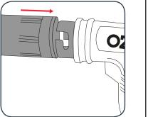
4 To lock into place, rotate nozzle in clockwise direction until nozzle clicks into place.
