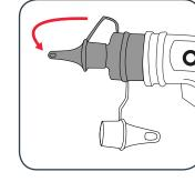
5 Fit small end of adaptor to the inlet on the device to be inflated. Once fitted, use On/ Off switch to inflate device.
