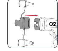
3 Connect inflation adaptor to the blower housing and rotate adaptor clockwise until it clicks into locked position.
