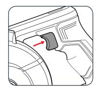
2 To stop the blower release the on/off switch.
