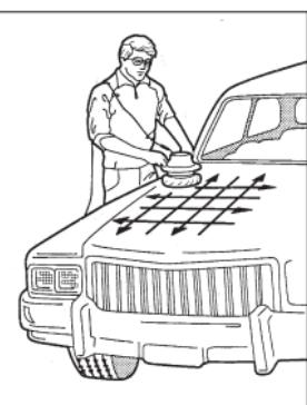
Now replace the textile polishing cap with the fine polishing cap and pull this over the polishing pad. Make sure it is completely clean. Remove the layer of polish in the same order as it was applied. **Important! Do not exert pressure on the polishing machine!**
