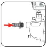
4. Securely attach the input hose or pipe (not included) to the other end of the adaptor. Ensure you have the correct diameter hose or pipe that is compatible with your water drawing source.
