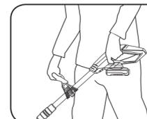
3. To turn on squeeze the on/off trigger whilst holding the lock-off button down.
