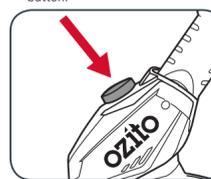
2. Tilt the cutter head to the desired angle.
