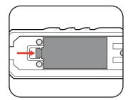
2 Insert 2 x AAA batteries in the correct direction indicated by the embossing inside the battery compartment.
