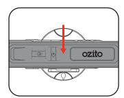
3 Use the dial on the bracket to adjust the height.
