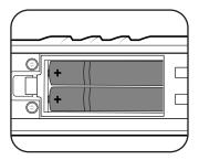
3 Place the side of the battery lid into the recess in the laser unit and push the lid tab down to secure in place.
