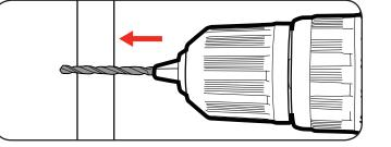
**Note:** Do not force the drill or apply side pressure to elongate the hole. Let the drill do all the work.
