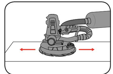
**Note:** It is recommended to keep the motor running for a short period of time after sanding, so that residual dust can be collected into the bag.
