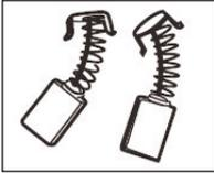
When the carbon brushes wear out, the sander will spark and/or stop. Discontinue use as soon as this happens. They should be replaced prior to recommencing use of the sander. Carbon brushes are a wearing component of the sander and are therefore not covered under warranty. Continuing to use the sander when carbon brushes need to be replaced may cause permanent damage to the
