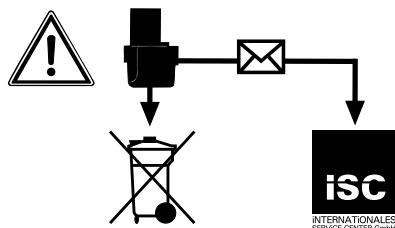
Rechargeable batteries and cordless electric machines and tools contain materials that are potentially harmful to the environment. Never place any cordless electric machines or tools in your household refuse. When cordless electric machines or tools become defective or worn, remove the rechargeable batteries and return them to iSC GmbH (address: Eschenstrasse 6, D-94405, Germany). If the rechargeable batteries cannot be removed, return the complete cordless machine or tool.
