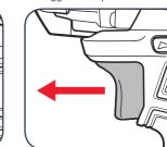
3 Control the speed by adjusting the amount of pressure applied to the
