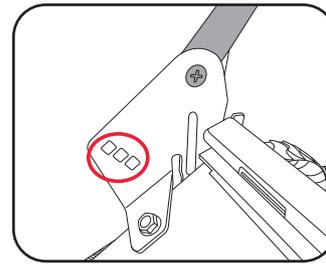
3. Fit the short round head bolt through the brackets and then through the lower handle. Secure each bolt with the 4 nuts and spanner provided.
