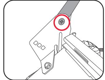
2. There are three holes remaining in each bracket, select the appropriate hole for the height of the user.
