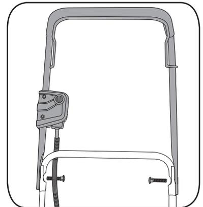
2. Secure knobs over the protruding ends of the bolts.
