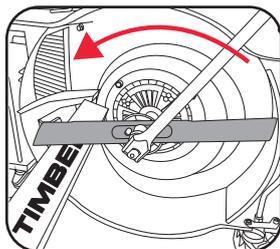
**Note:** A piece of timber will assist in holding the blade while removing or tightening the blade bolt.
