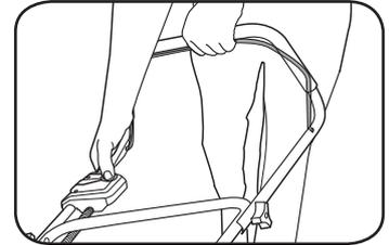
3. Release the start/stop motor lever to stop the mower.
