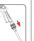
WHEN RELEASING THE QUICK-RELEASE COUPLING, BE SURE TO HOLD THE COUPLING PIECE TO PROTECT YOURSELF AGAINST INJURY FROM THE REBOUNDING HOSE.
