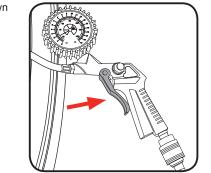
6. After a short time, release the trigger and check the tyre pressure by referring to the pressure gauge.
