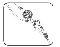
2. When inflating tyres with normal "Schrader" valves, no adaptors need to be fitted to the rubber hose.
