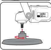
3. To remove the accessory disc, press and hold down the spindle lock button, then turn the accessory disc clockwise to unscrew it.
