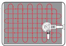
**Note:** Start at the lower speed settings and slowly increase the speed as required within the recommended settings. Use only speeds 5, 8, & 10 for polishing applications to prevent damage to the surface.
