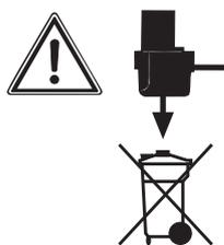
Rechargeable batteries and cordless electric machines and tools contain materials that are potentially harmful to the environment. Never place any cordless electric machines or tools in your household refuse. When cordless electric machines or tools become defective or worn, remove the rechargeable batteries and return them to iSC GmbH (address: Eschenstrasse 6, D-94405, Germany). If the rechargeable batteries cannot be removed, return the complete cordless machine or tool.
