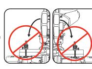
**WARNING!** ENSURE THE MATERIAL IS SECURELY CLAMPED BEFORE MAKING ANY CUTS. FAILURE TO SECURE THE MATERIAL MAY CAUSE THE WORKPIECE TO FLY OFF AND CAUSE PERSONAL INJURY.
