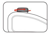
2. Fill the media container with suitable sand blasting media. Screw the lid onto the container to secure.
