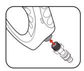
4. Pull back the sleeve on hose fitting, insert male end & release sleeve on hose fitting.
