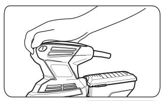
3 Let the motor build up to maximum speed. Gradually lower it onto the workpiece with a slight forward movement.
