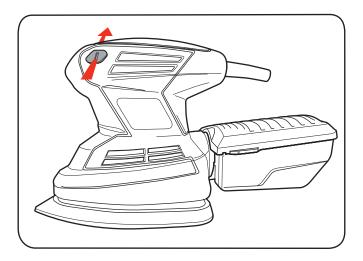
3 To turn off, press the 'O' button into the housing.
