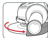
WARNING DO NOT OPERATE THE ANGLE GRINDER WITHOUT THE SAFETY GUARD FITTED AS POSSIBLE INJURIES COULD OCCUR.
