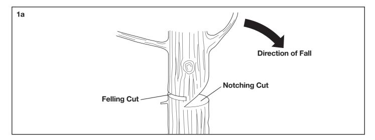
Felling is the type of cut used to cut down trees. Whereas it may be possible to cut down small trees (6-7 inches in diameter) with a single straight through cut, larger trees require a felling cut.
