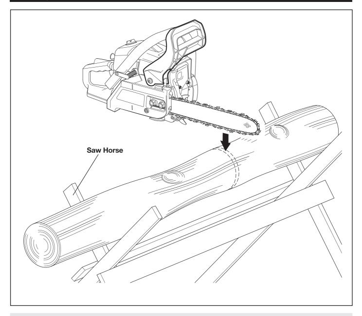
A bucking cut is used to cut a fallen or felled tree into small manageable lengths or logs. Usually the tree trunk will be supported at one end, both ends or along its entire length. Often this type of cut is performed using a sawhorse which provides all the required support to keep the trunk stable.
