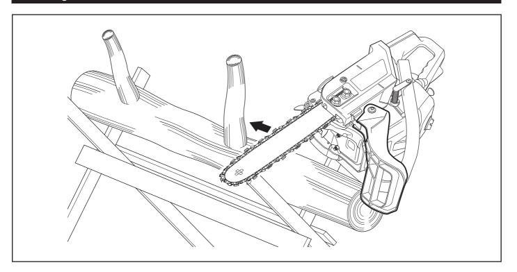
This type of cut is used to remove small branches from a felled or fallen tree. Cuts can be made horizontally or vertically to the bottom of a branch. Usually limbing cuts are performed when a tree trunk has been cut into small manageable lengths using a bucking cut. Branches under tension should be cut from the bottom up to avoid binding the chainsaw.
