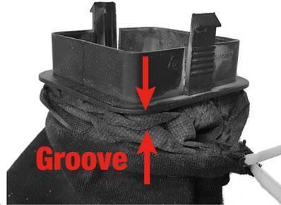
3. Overlap the cable tie around the opening all the way around the adaptor, ensure the cable tie sits within the groove around all four sides.
