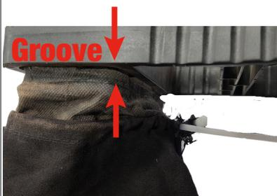
3. Overlap the cable tie around the opening all the way around the adaptor, ensure the cable tie sits within the groove around all four sides.
