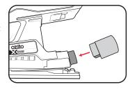
3. Push the adaptor firmly into the port and attach a vacuum hose to the other end.
