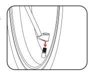
5 After a short time, release the air chuck and check the air pressure with the pressure gauge.
