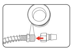
2 Insert the 1/4" male nitto quick plug of the air hose into the quick-lock coupling of the air compressor by pulling back the sleeve and inserting the plug.
