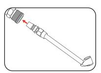
2 The tyre chuck included in this kit is made for "schrader" valves.
