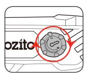
2. To lower the temperature rotate the temperature control dial anti-clockwise.
