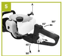
Important: The cutting blades will start to work when the engine starts because the throttle lever is locked. Then release the throttle lever by simply pressing it (the engine will return to idling speed).
