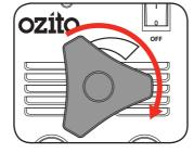
2 To decrease the welding current turn the current regulating knob in a anticlockwise direction.
