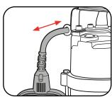
**NOTE:** There must be a minimum of 100mm of cable from the adjuster to the float.
