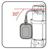
3. To set the pump to switch off at a higher water level, adjust the float switch cable length in the adjuster.
