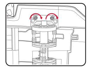
4. Refit and tighten the two socket head screws.
