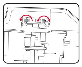
1. To remove the roller, first remove the two socket head screws. Put aside for later use.
