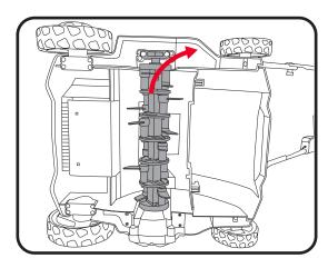
2. Lift the roller at this end and pull it out, away from the scarifier.
