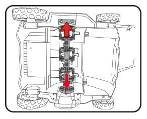
3. To fit the roller, first push the roller in the square-ended drive, then push the other end into the scarifier.
